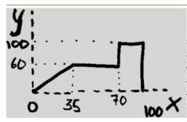
Here is an example of a simple drawing, some outline of something we want to have as a series of lines on our paper. In user coordinates the x varies from 0-->100, and y also 0-->100. All of HP's HP-GL plotters have a hardware resolution of 40 increments per millimeter, which constitutes the absolute increments. A reletive movement of 8000
